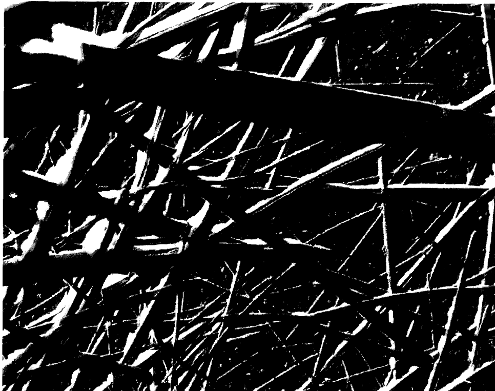
Figure 3 Area of numerous lath crystals, after polymerization at 170°C for 3 h, followed by annealing at 400°C for 30 min
